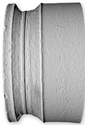
9 mm CC surface 1 FOV rim. Stripe width: 5.8 mm Scan time: 9 min File size: 82 MB
